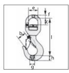
Safety hoist hook LKNK type same as LKN, but swivel with ball bearing
