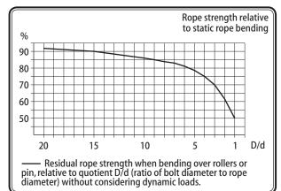
The bend diameter should, depending on material and construction, be adequately large, certainly no less than 5d for fibre ropes made from polypropylene, polyamide and polyester; 8d for wire ropes made from polyamide (d=nominal rope diameter). In ropes made from high modular polyethylene or aramid the bend radius primarily depends on the rope construction, therefore the manufacturer or supplier should be consulted. Sharp edges must at all times be avoided, if necessary by using edge protection.
