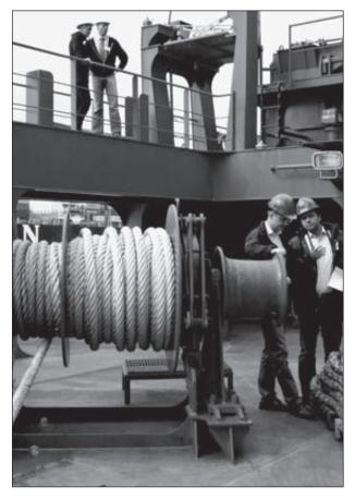
Hence the positioning and specifications of winch drums, rollers and chocks must satisfy requirements of mooring ropes in terms of size, flex, dynamic load properties and material. Efficiency and life of ropes depend critically on how rope guiding equipment and winches, in particular automatic winches, are conditioned, controlled and maintained. In view of the large (almost confusing) variety of synthetic ropes on offer today, it makes sense to break down into categories:
