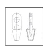
**Lig type rope socket** Highly wear-resistant cast steel to DIN 17182 Nom. size 2 to 15 for rope diameters 11 to 48mm
