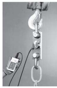
LL Link with remote display for robust use, measuring range 0-2,000 kg to 0-75,000 kg
