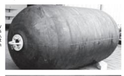
with foam filling, PU coated surface, optionally with chain-tyre net jacket for extra surface protection
