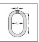
WLL figures shown refer to single leg use. Chain diameters shown refer to use with grade 80 lifting chains.
