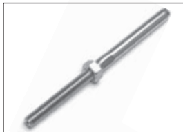
Screw end swage terminal with nut Material: AISI 316 Finish: high gloss polished Rope dia. 2,5 to 16 Thread M 5 to M 16
