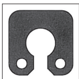
Solid rubber fender in round-, square-, D- or U-profile
